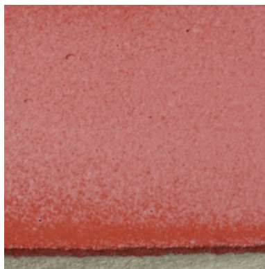
Fig. 2 Skim Coat without ERASEAL120 after testing with strong efflorescence and no hydrophobic properties
